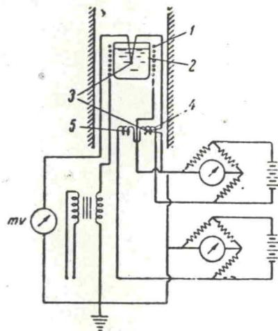
Fig. 1. Circuit diagram for measuring the melting points of metals at ultra-high pressures.
