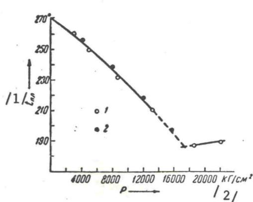
Fig. 2. Melting point of bismuth as a function of pressure.
